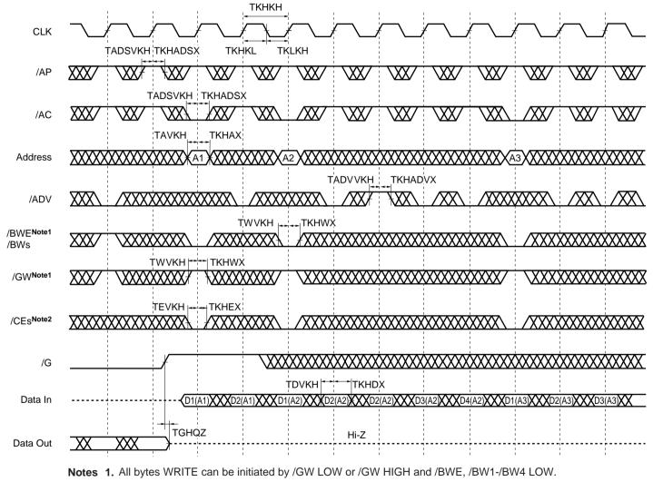
/CEs refers to /CE, CE2 and /CE2. When /CEs is LOW, /CE and /CE2 are LOW and CE2 is HIGH. When /CEs is HIGH, /CE and /CE2 are HIGH and CE2 is LOW.
